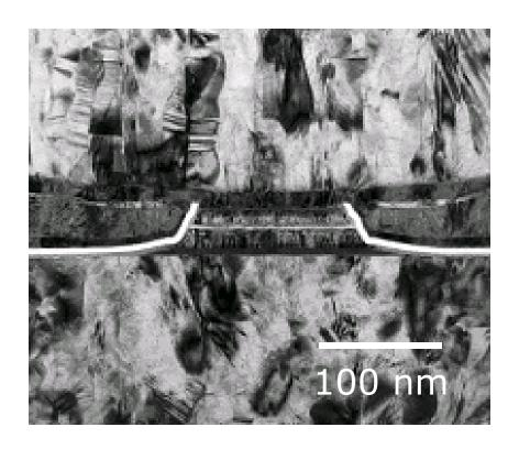
TEM micrograph of tunneling magnetoresistive sensor (view from "air bearing side") M. Kautzky (Seagate)
